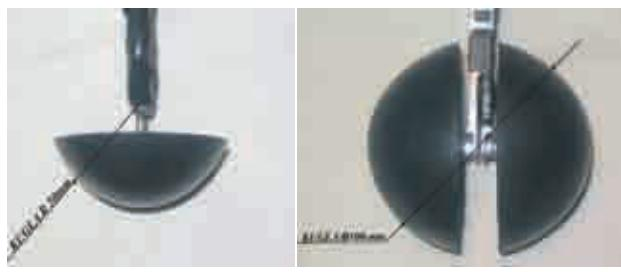
Figure 4. Physical models of the head (a) and epicranium (b)
