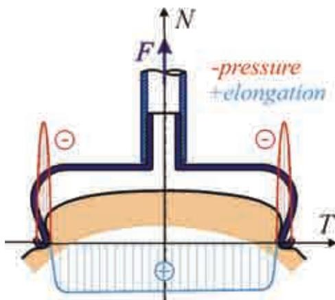
Figure 10. Stress zone prior to angular tractions.
