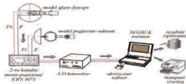
Figure 5. Metrical system scheme for model of head extraction by forceps and vacuum.
