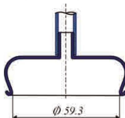
Figure 11. Calotte diameter defining the vacuum zone.
